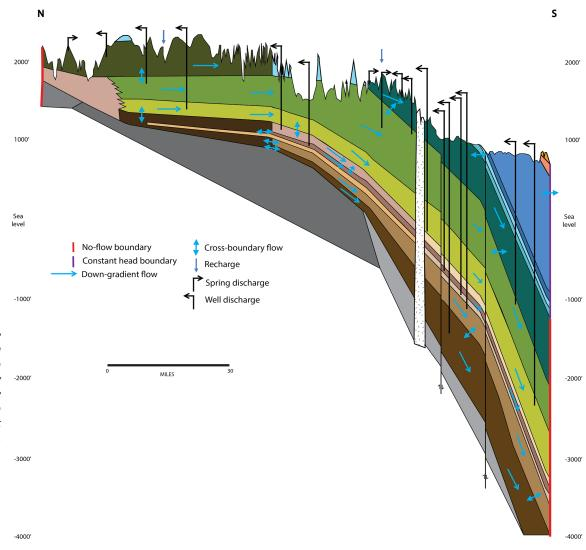
This figure represents the hydrologic dynamics in a given system, with recharge, cross-boundary flow, and discharge regimes specified with respect to geologic formations.
