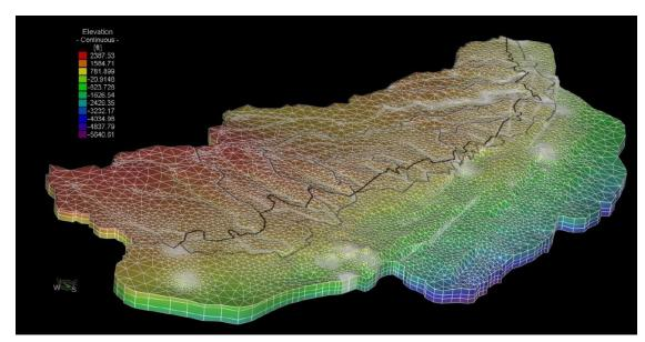
An example of a numerical model for an aquifer system
