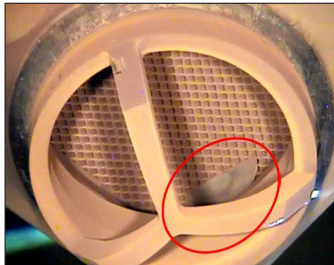
Foreign Object Removal Through Ultrasonic Cleaning
