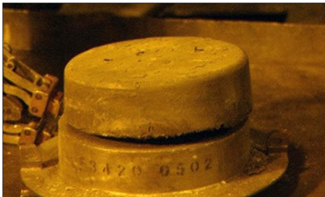
EMT-derived HALEU in the form of 30–40 kg ingots (top left) are recast in a multi-tier crucible system (top right) to yield 1.5–3 kg fuel fabrication-ready reguli (bottom right).
