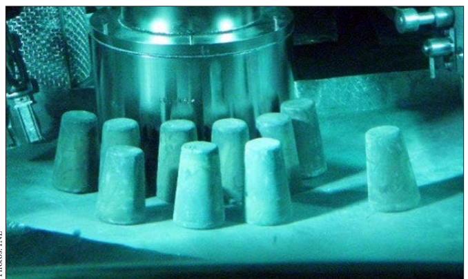
EMT-derived HALEU in the form of 30–40 kg ingots (top left) are recast in a multi-tier crucible system (top right) to yield 1.5–3 kg fuel fabrication-ready reguli (bottom right).
