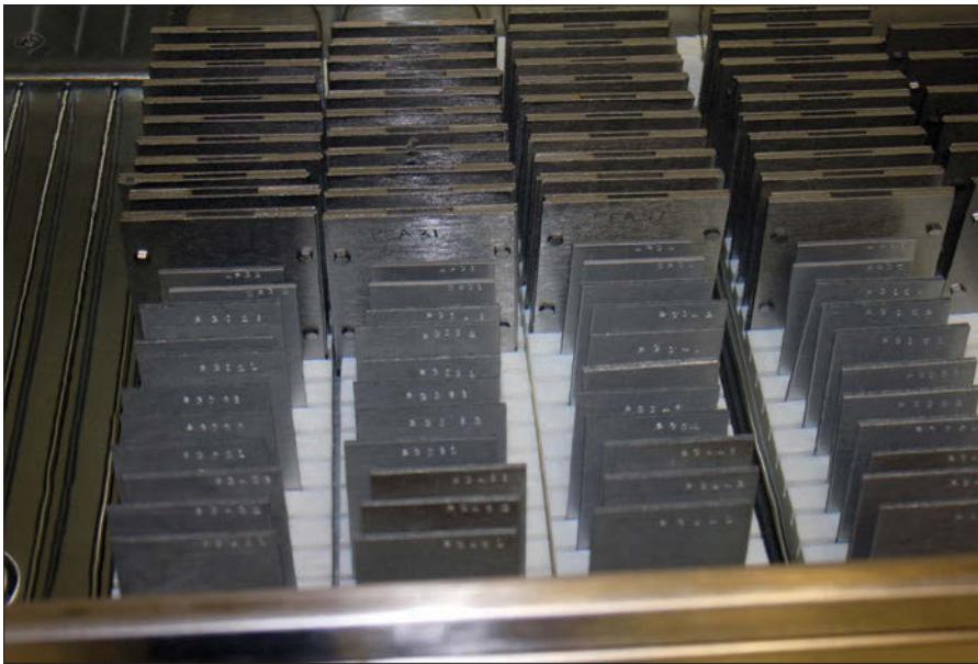
Fig. 2. BORAL coupons set in a test bath.
